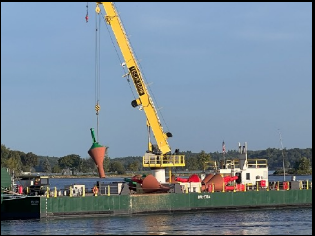
Barge crane lifting a new buoy into place.
